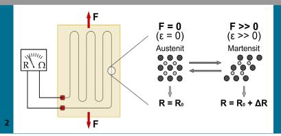
Glass fiber reinforced plastic with integrated strain sensor based on SMA wires
