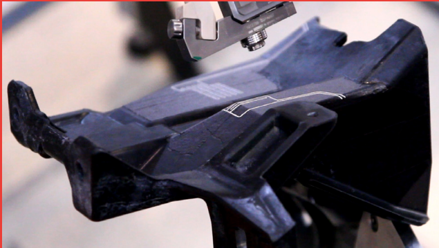
1 Functionalization of headlamp frame 2 With LEDs and conductor tracks functionalized aluminum-component
