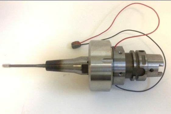
1 Ultrasonic vibrational system with drill, heat-shrink holder and HSK63 fitting
